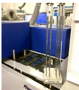
Fig. 1. Reactors Assembly of high throughput reaction.
